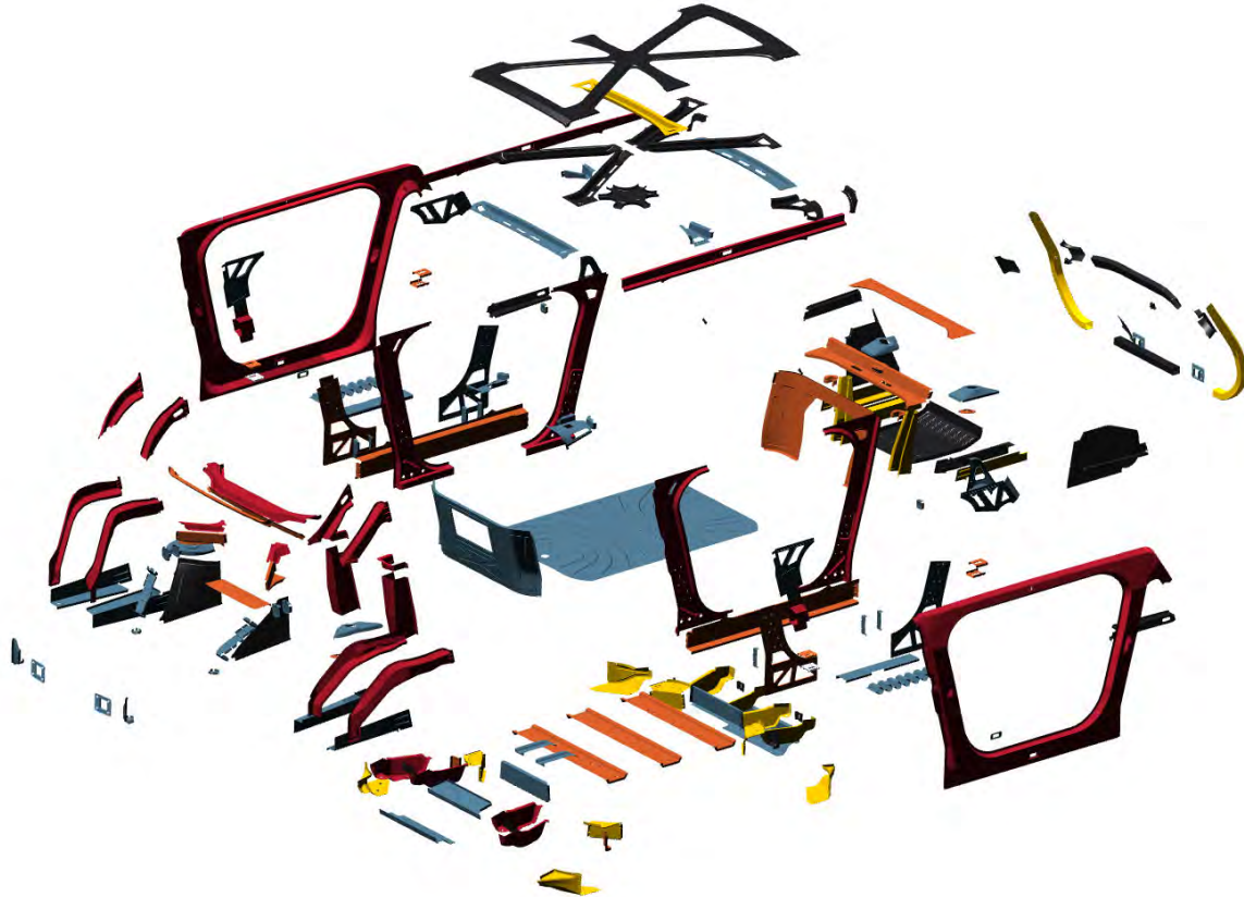
Figure 7.2.1.4 Steel E-Motive SEM1 BIW AHSS grades (exploded view) (See Appendix 4 for larger image)
