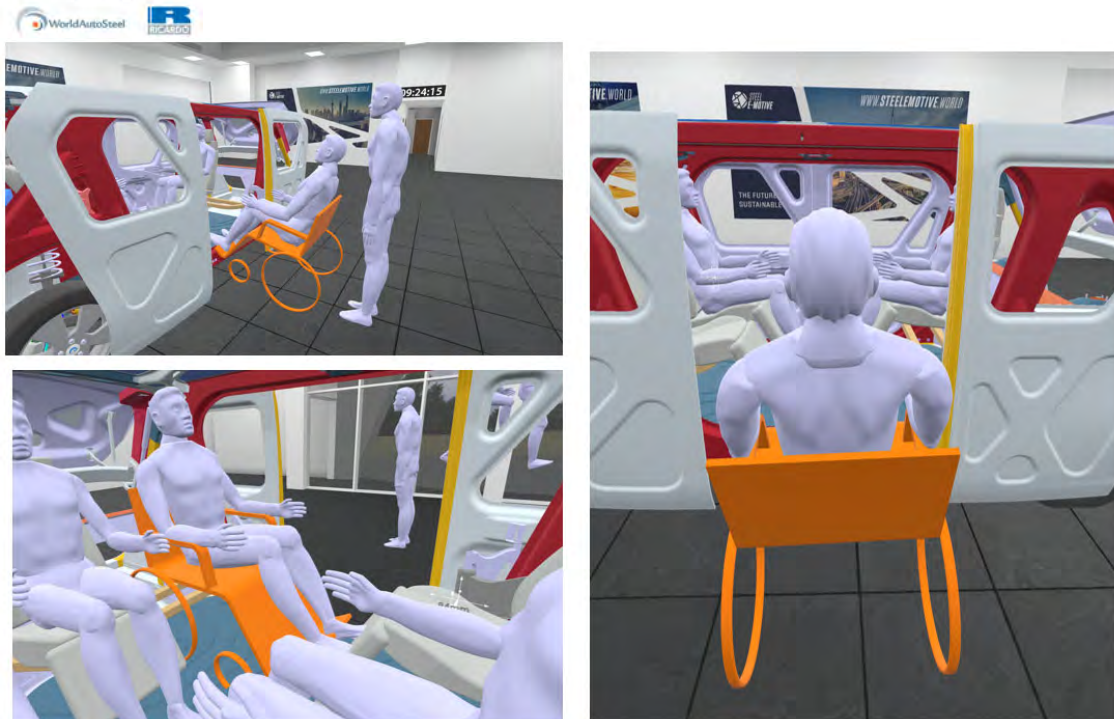
Figure 7.1.4.1 SEM1 wheelchair user vehicle access evaluation using Virtual Reality tools
