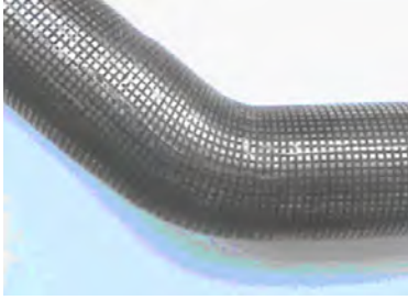
Figure 5.6: DP 590 formed into a tube w/45 degree bend, then laser welded.
