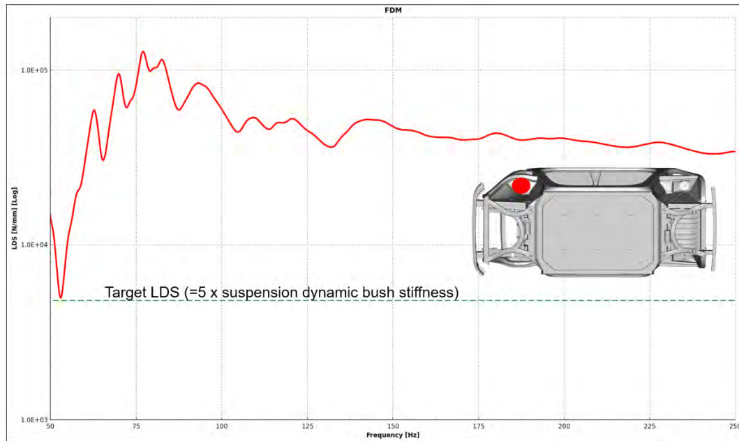
Figure 7.2.2.8 Local Dynamic Stiffness (LDS) of front damper strut top (trimmed BIW FE analysis)
