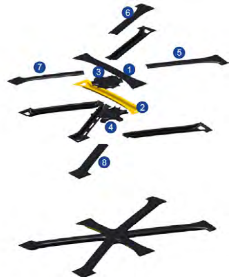
Figure 7.2.5.19 SEM1 mid zone roof structure and AHSS grades (See Appendix 4 for larger image)
