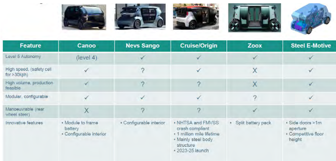
Figure 6.2.4.1 High level specifications and features of comparable vehicles to Steel E-Motive. (Data sources: https://www.canoo.com/ https://www.nevs.com/en/pons/ https://getcruise.com/ https://zoox.com/vehicle/ ) Information believed to be correct at the time of writing.
