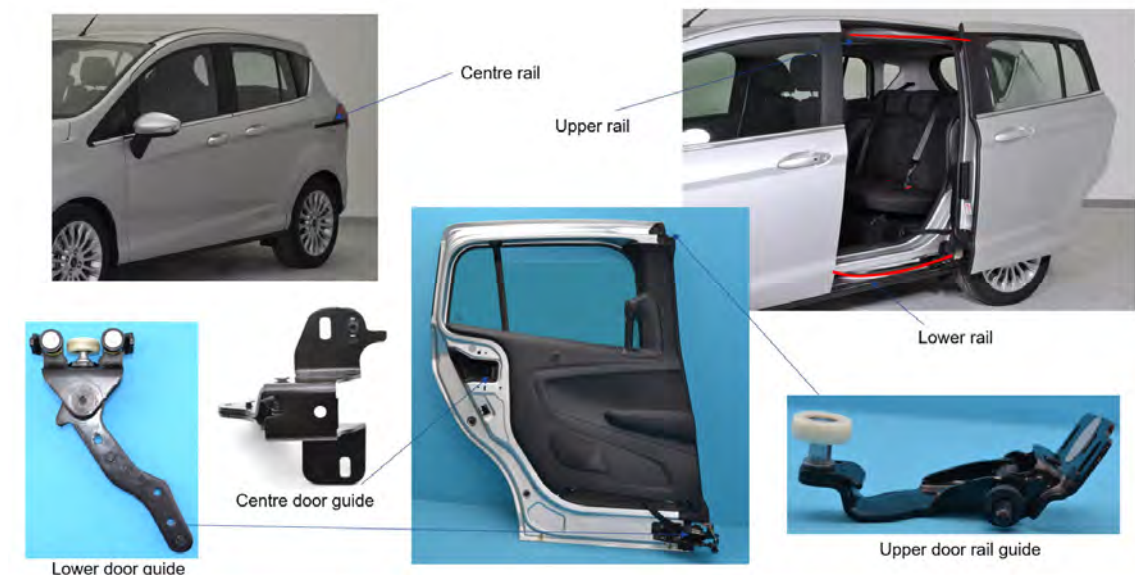
Figure 6.3.5.1.1 Track and rail sliding door, Ford B-Max passenger car (images from a2mac1)
