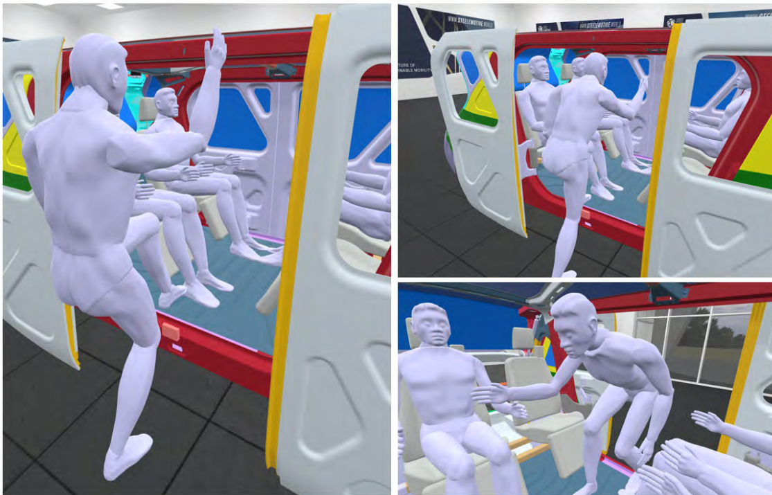
Figure 7.1.3.2 SEM1 occupant ingress and egress study (95 th percentile male) using Virtual Reality tools
