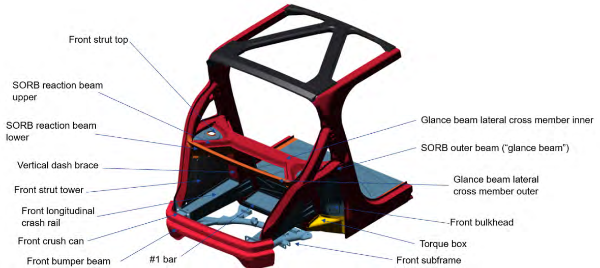
Figure 7.2.3.1 Primary subassemblies in SEM1 front crash structure (See Appendix 4 for larger image)
