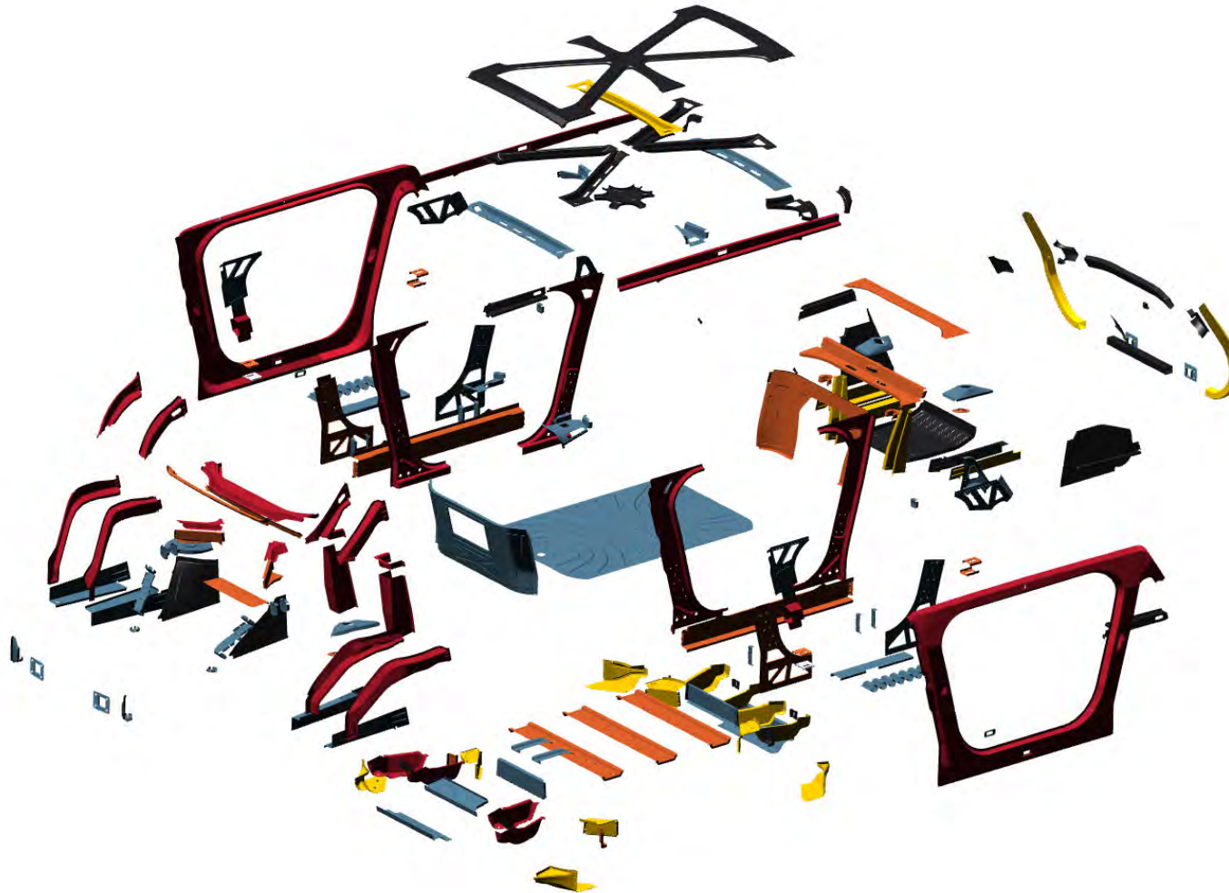
Figure 7.2.1.4 Steel E-Motive SEM1 BIW AHSS grades (exploded view)
