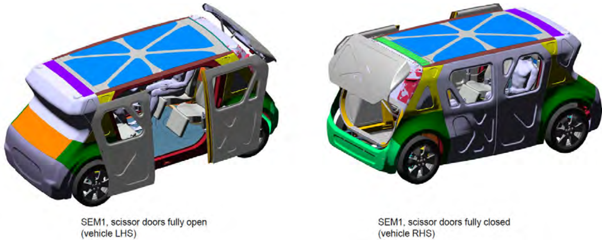
Figure 7.4.1.2.1 SEM1 scissor doors – open and closed positions
