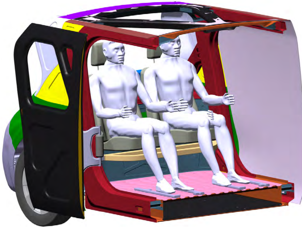
Figure 7.1.2.1 SEM1 engineering 3D CAD model, section cutaway in X, looking to the front of the vehicle showing front occupant (95 th percentile mannequins) in rear facing, front seat configuration. Occupants are positioned where conventional vehicle controls would be located. (doors in open position).
