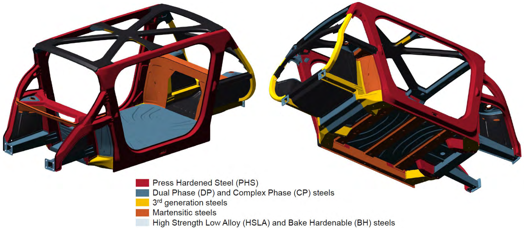
Figure 7.2.1.1 Steel E-Motive SEM1 BIW design and distribution of AHSS
