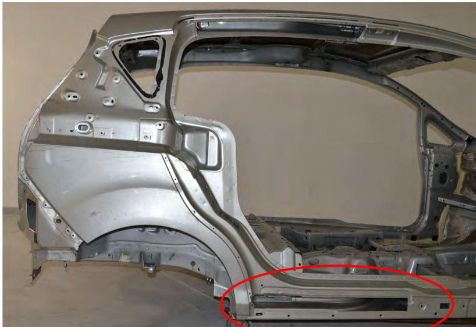
Lower rail, encroaching into rocker space
