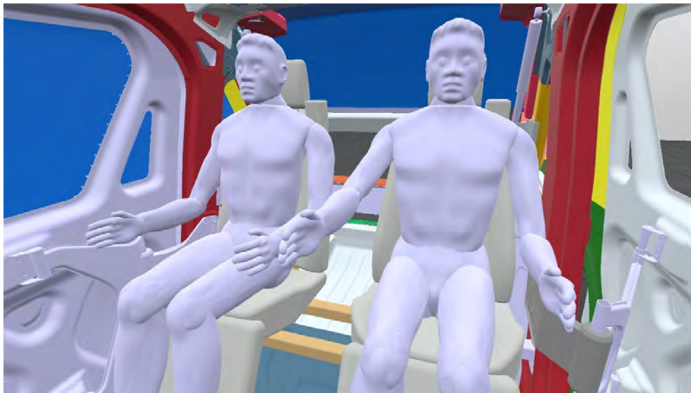
Figure 7.1.3.4 SEM1 interior space evaluation using Virtual Reality tools
