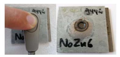
Figure 125: Orientation of probe on specimens.
