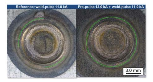
Figure 6-28: Experimental results of main-trials for pre-pulse welding schedule for MTC DP1200 - thick mild steel (2.00 mm)
