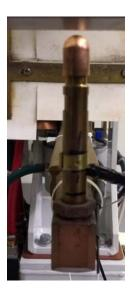
Figure 142: Lower electrode where the transducer is imbedded.
