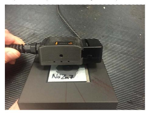
Figure 46: New Padded ECA probe developed in this project for RSW.
