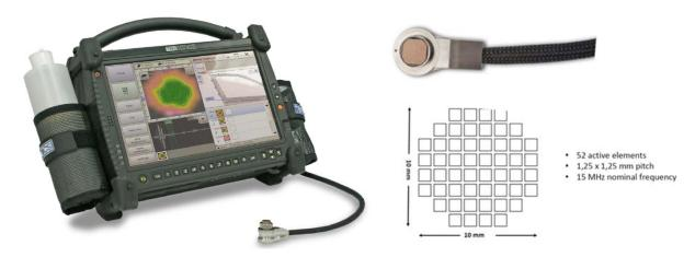
Figure 123: RSWA System (left) and zoom on probe (right).
