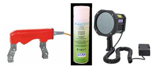
Figure 30 : Electromagnetic yoke (left), Magnetic liquid (middle), UV lamp (right).
