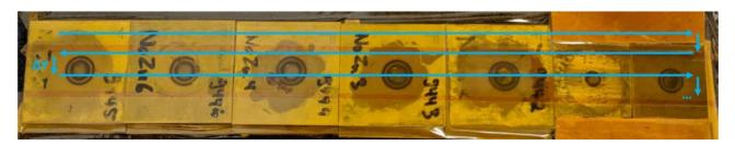
Figure 43: Representation of the path carried out by the XY table on the samples studied. A kapton tape placed above specimens to facilitate probe movement.
