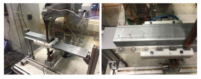
Figure 16: AE monitoring of closed hat profile.
