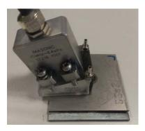
Figure 57 Phased array probe positioned laterally from the spot weld.
