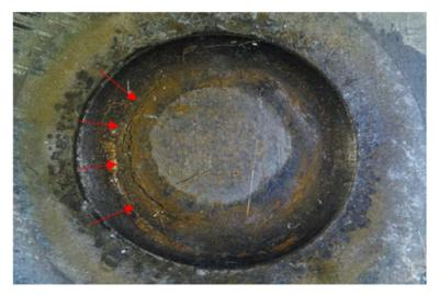
Figure 139: LME crack obtained at 1200ms and 8.4kA.
