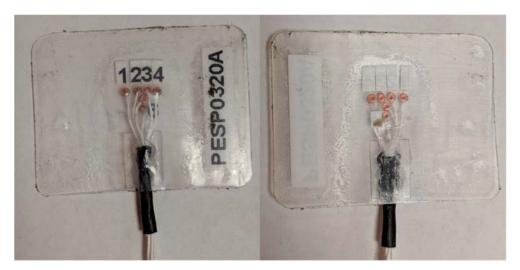
Figure 44: Example of assembly of test coils. On the right we have the face of the top and on the left the face of the bottom which will be in contact with the spot weld.
