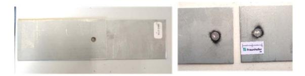
Figure 6-63: Calibration shear tensile specimen.
