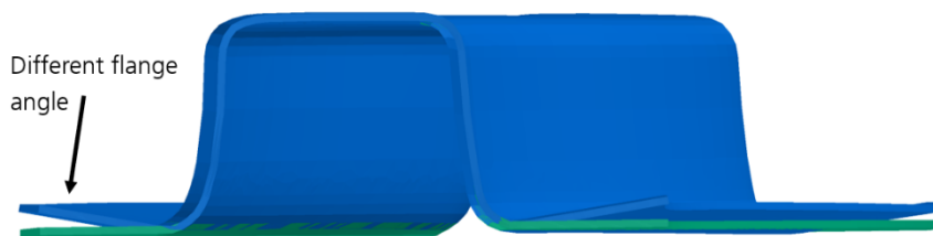
Figure 5-6: Straightened (green) and springback-afflicted (blue) geometries.
